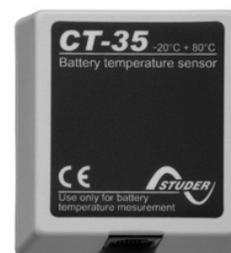
Operating voltage of lead-acid batteries change depends on the temperature. To correct the operating voltages according to the actual temperatures, a temperature sensor can be connected to the COMPACT.
