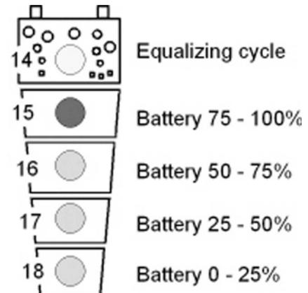
This means that the display can, within few minutes during the charge, commute from 25% to 75% or during the discharge, to the opposite direction.
