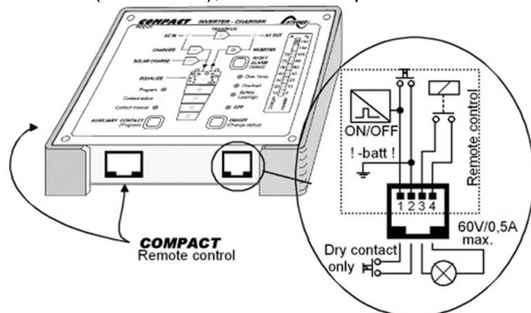
**Caution: No external voltage should be connected to this Input Control.**
